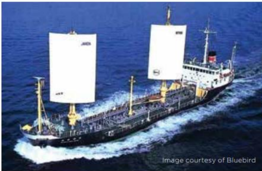
Vessel Shin Aitoku Maru with rigid sails
